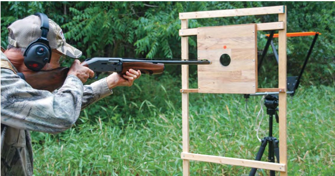
Chronographing shotshells is important for assessing the loads. The author devised, built, and used a special setup as described in this report. High Gun produced fantastic results in this assessment.
