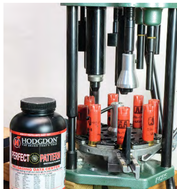
Due to the fine granulation of Perfect Pattern, charges were dispensed by this RCBS Grand progressive loader with very little variation in weight.
