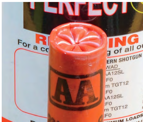
Correct stack height of powder charge, wad, and shot charge specified by a ballisticians along with proper adjustment of the crimp die and wad seating pressure of the loading press by its operator result in crimp quality accurately described by a single word—perfect.
