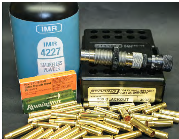
Subsonic handloads can be very accurate. For example, IMR 4227, Remington 7½ primers, Starline cases, and Redding dies produce excellent 300 Blackout ammunition.
