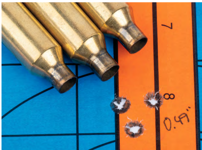
Several cartridges showed a distinct liking for Ramshot Grand during the author's accuracy tests. This is a typical 100-yard group produced by the 6.5 PRC and Hornady 147-grain ELD Match bullets.
