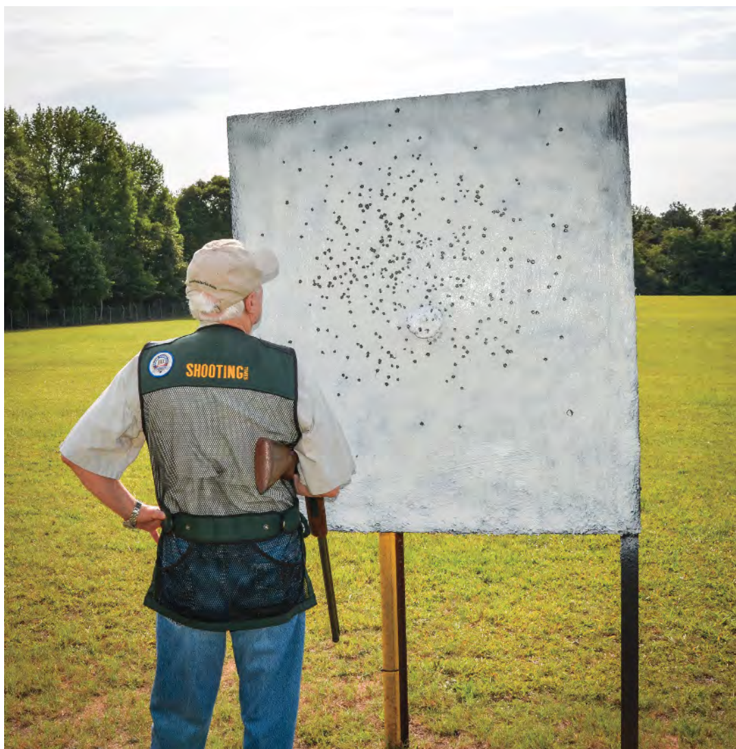
Layne uses a steel plate to pattern-test shotguns at various distances. The performance of loads containing Perfect Pattern powder proved to be quite good.
