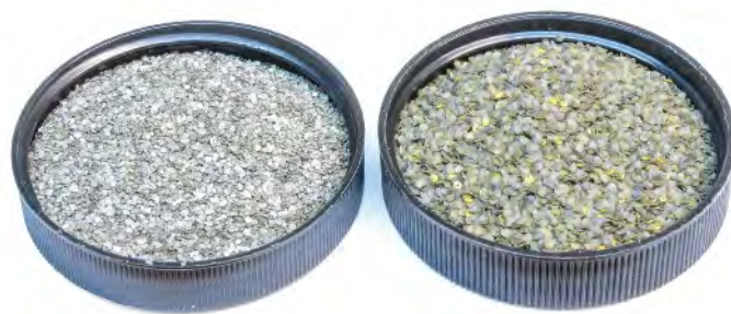
Perfect Pattern (left) and Clays are double-base propellants deriving their energy from a mixture of nitrocellulose and nitroglycerine. Due to its smaller granulation, Perfect Pattern is denser.
